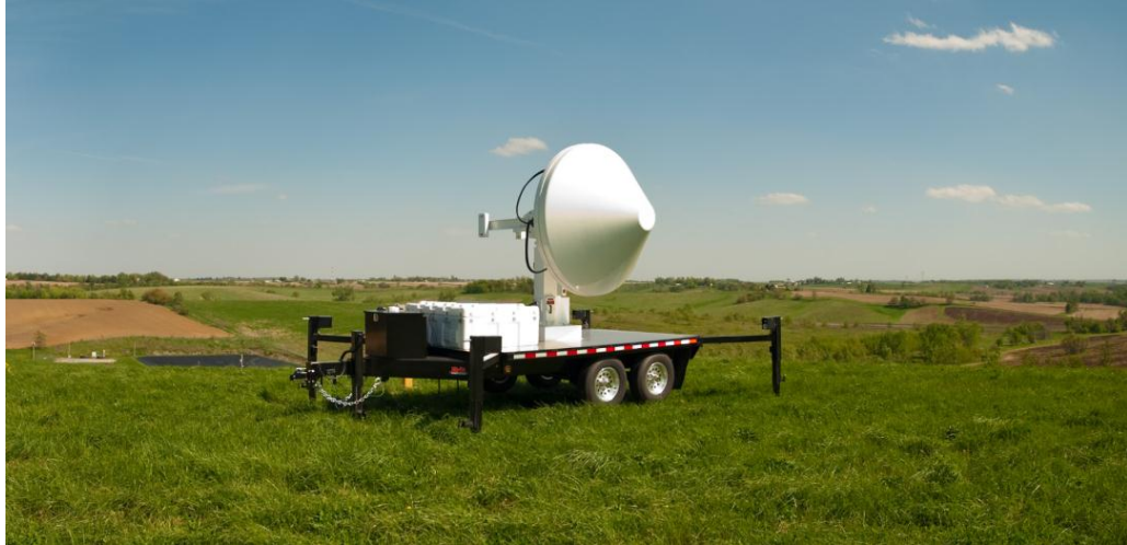
Figure 4.1: X-band polarimetric radar network node at Iowa City landfill.
